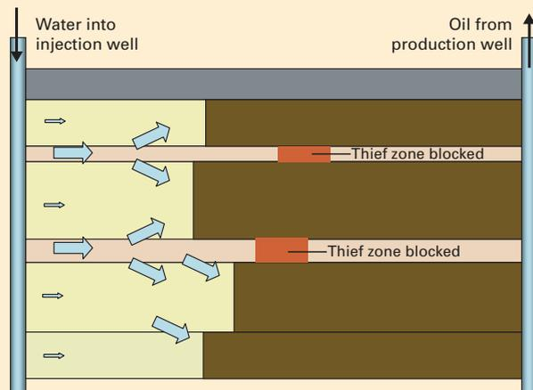
**Solution:** Bright Water particles are injected along with the water and ‘pop’ in the warmer sections of the thief zones. This blocks the thief zones and redirects water to poorly swept oil-bearing zones, recovering more oil from the reservoir.
