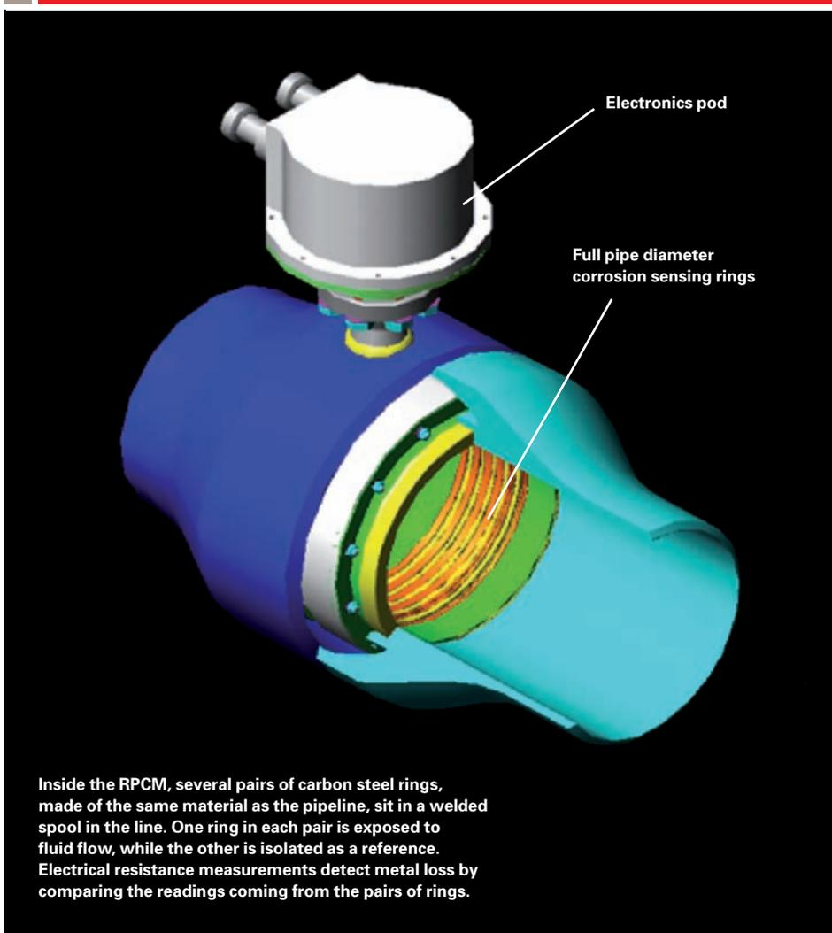
**Inside the RPCM, several pairs of carbon steel rings, made of the same material as the pipeline, sit in a welded spool in the line. One ring in each pair is exposed to fluid flow, while the other is isolated as a reference. Electrical resistance measurements detect metal loss by comparing the readings coming from the pairs of rings.**
